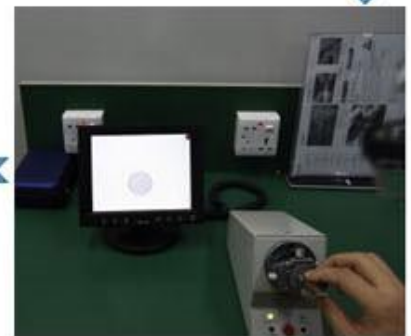
Cleaning end face
